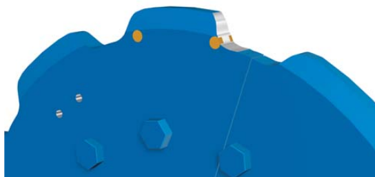
Tooth profile wear and indicator pins
